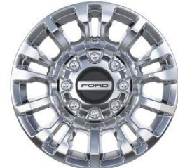
18" Chrome PVD Aluminum (included in XLT Premium Pkg. (17P), Chrome Pkg. – (17C)) – 647
