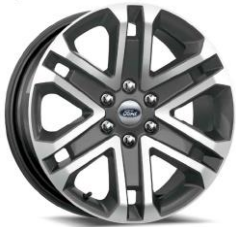
20" six-spoke machined aluminum with Magnetic painted pockets (Opt. w/ STX Appearance Pkg) – 642
